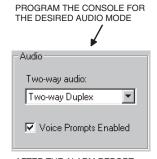
AFTER THE ALARM REPORT IS SENT, THE CONSOLE WILL SWITCH TO THE PROGRAMMED AUDIO MODE FOR 90 SECONDS CENTRAL STATION OPERATOR:
